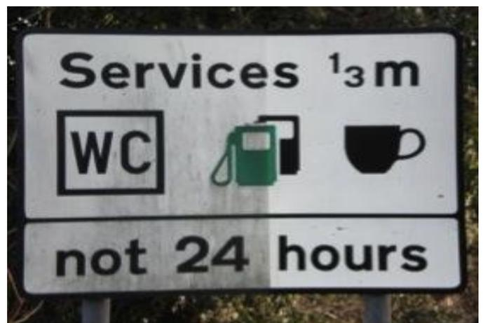
Photocatalysis results after three years on a road sign
